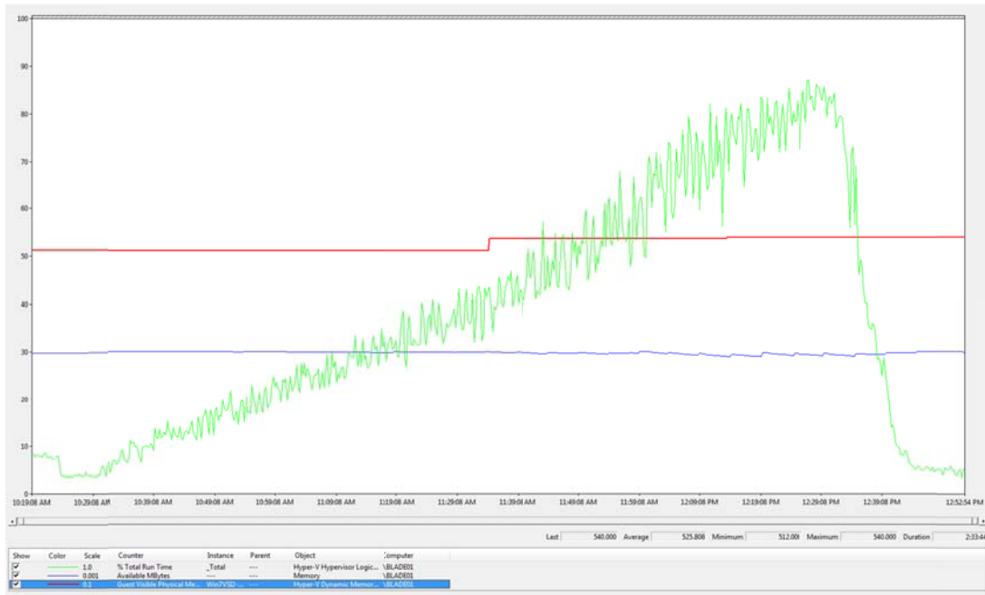
Figure 5: Perfmon log for a test of 120 Windows 7 SP1 32-bit guests.
